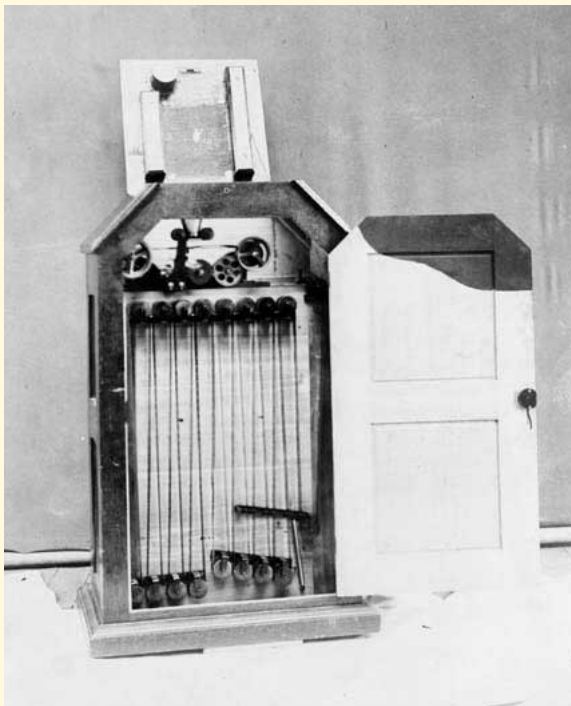
Edison's Kinetoscope , open. Film was threaded on rollers as a continuous ribbon.
